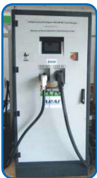
100 kW DC Fast Charger Technology
