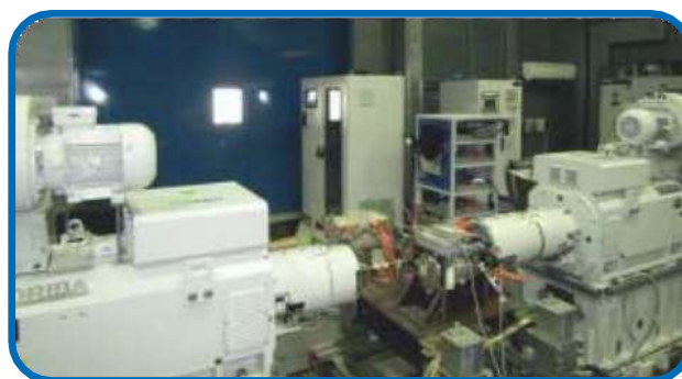
Machine-in-Loop setup for Vehicle Components Testing
