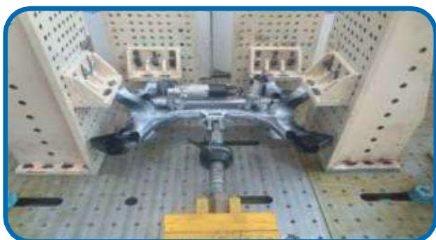
Static Stiffness and Strength Testing of Front and Rear Sub-frames
