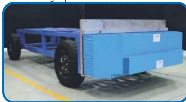
Mobile Barrier Trolley as per Euro-NCAP Protocol
