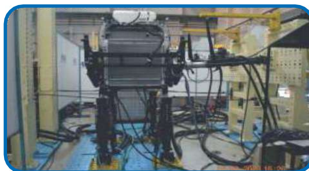
Multi-axial Durability Testing of Cooling Module Assembly
