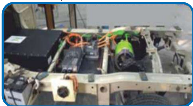
Developed E-axle fitted on 1.5T SCV
