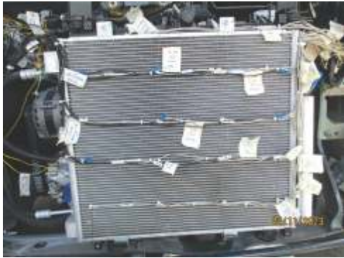
Temperature and Airflow Measurement Grid on AC Condenser
