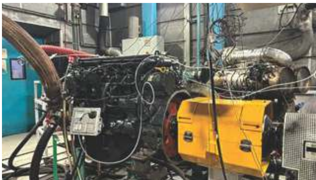
Engine Test Bed Setup
