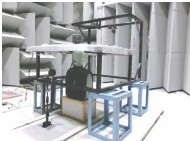
Sound Quality Assessment of Electric Vehicle Sunroof Assembly
