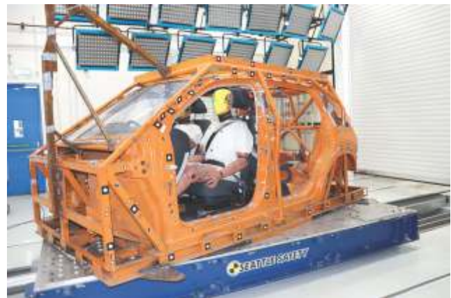
Advanced Acceleration Sled Test Facility
