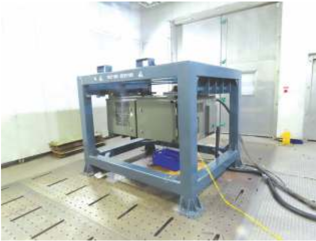
Performance Verification of Railway Compressor
