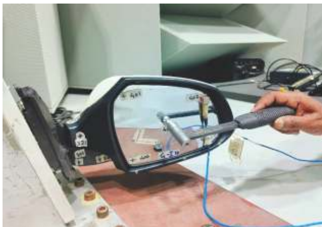
Experimental Modal Testing of Door Mirrors
