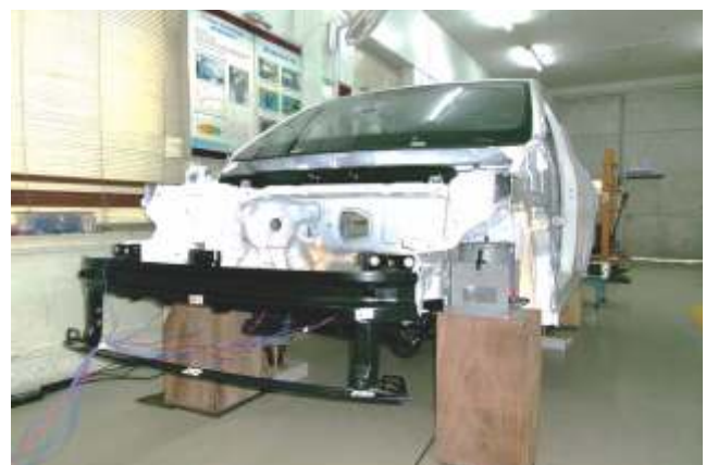
Torsional Dynamic Stiffness Evaluation of BIW
