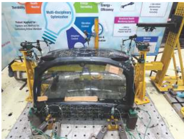
Tailgate Stiffness Measurement
