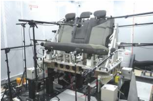
BSR Noise Evaluation of Driver and Rear Seats
