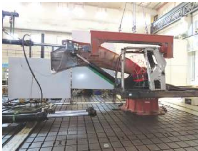
Roll Over Protective Structure (ROPS) Test as per ISO 12117-2
