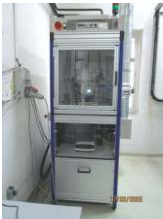
Canister Ageing Bench for Fuel Vapour Ageing
