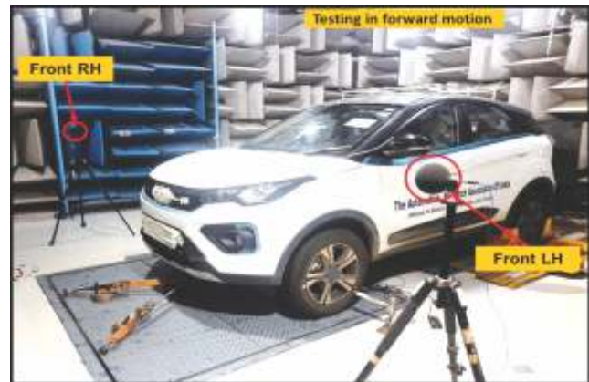
Integration of AVAS unit in an EV
