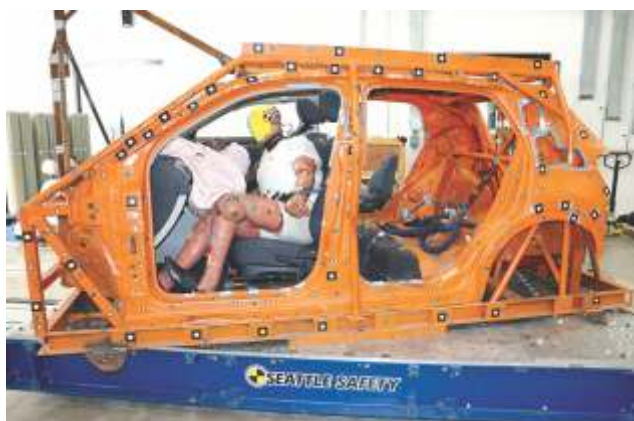
Knee Mapping Sled Test
