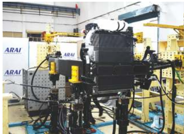
Structural Durability Testing of Cooling Module Assembly
