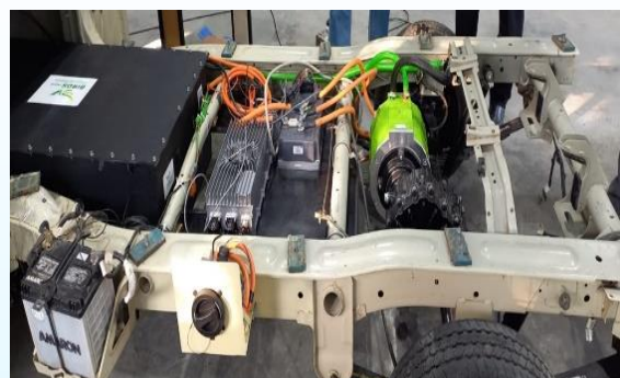
Fig.3: Indigenously Developed E-Axle Based Powertrain for Small Commercial Vehicle
