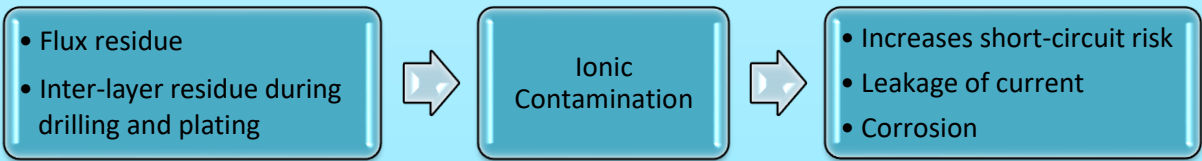
Fig. 1: Sources and Effects of Ionic Contamination
