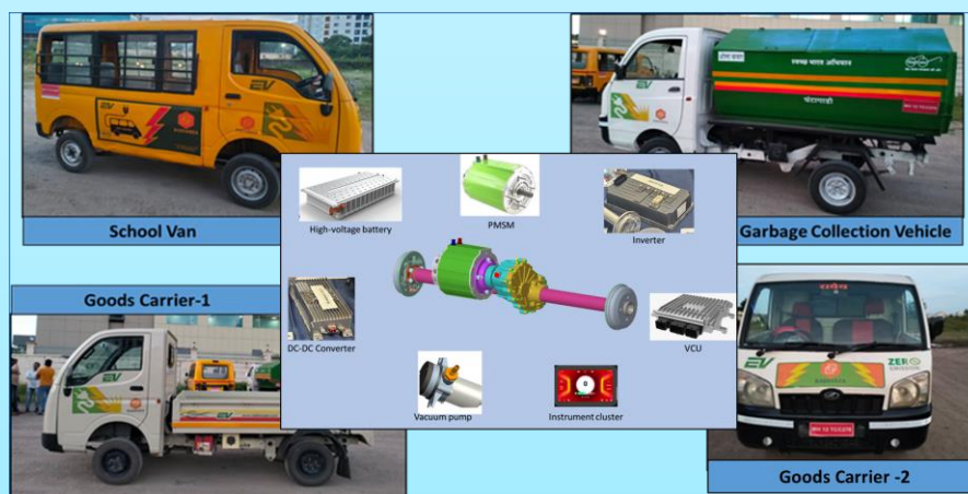
Fig. 4: Fleet of SCV (1.5 Ton GVW) Running with Retrofitted E-Axle Powertrain
