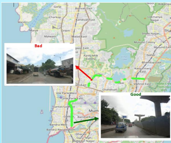
MARG 2.0 Application – Road Roughness data along with Geo Tagged Photograph
