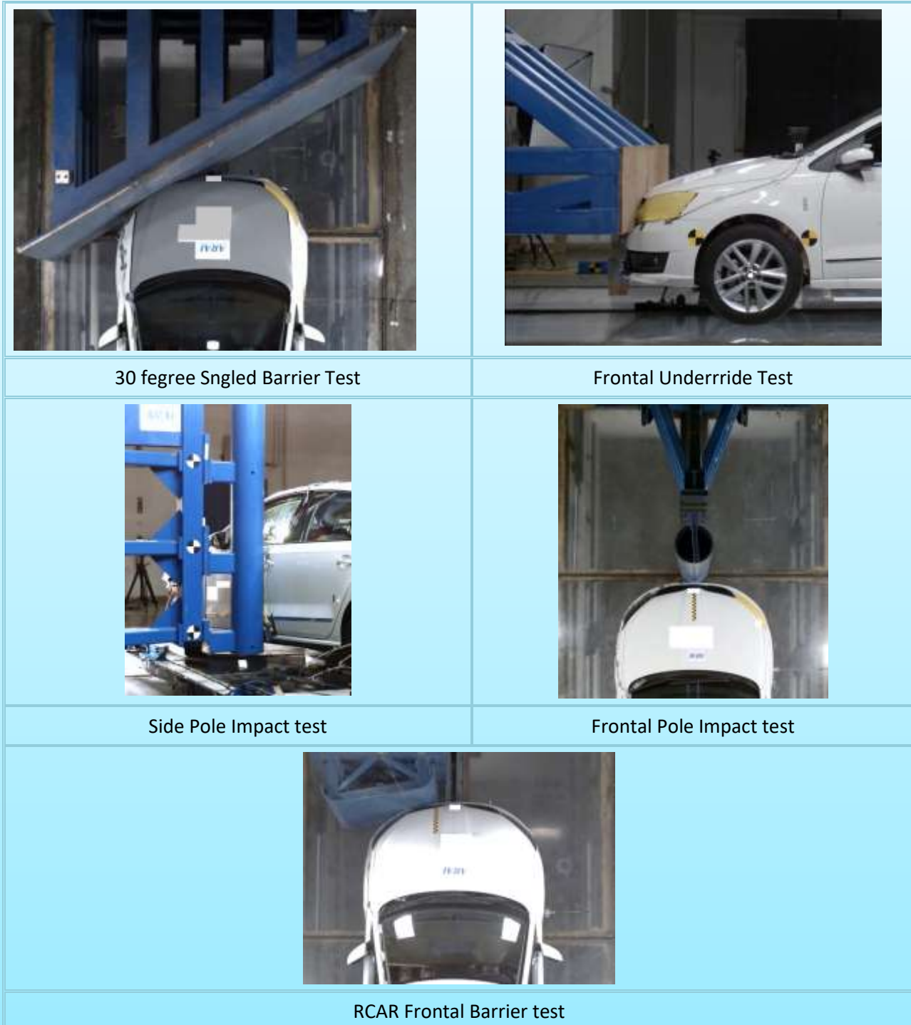
Fig. 9 : Various test configurations for development and modifications of frontal and side airbag algorithm
