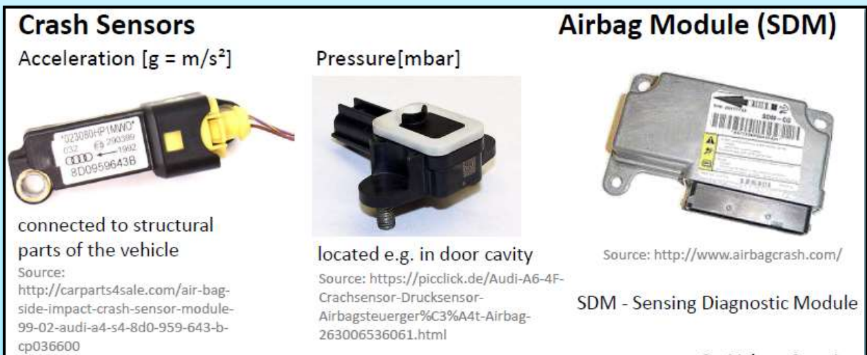
Fig. 4 : Crash Sensing System components
