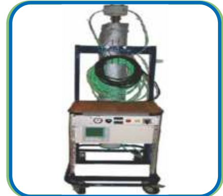
Ammonia Measurement System from Engine Exhaust
